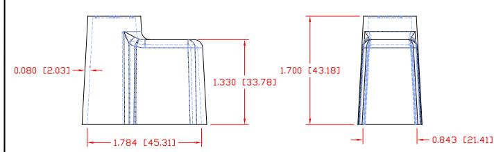
SCALE FACTOR : NONE ALL DIMENSIONS GIVEN AS: in [mm] TOLERANCES UNLESS OTHERWISE SPECIFIED : MOLDED PARTS: ±.030" [±0.8mm] ALL ANGLES ARE ± 1 DEGREE
